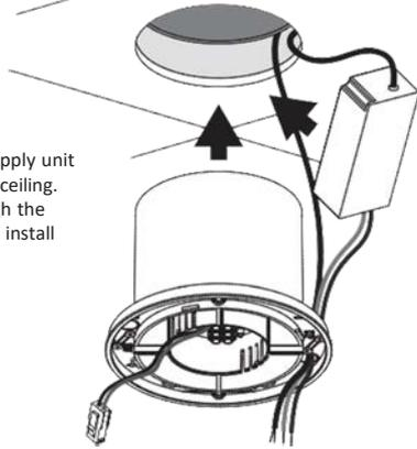
Fix the fan on the ceiling surface using the screws.
