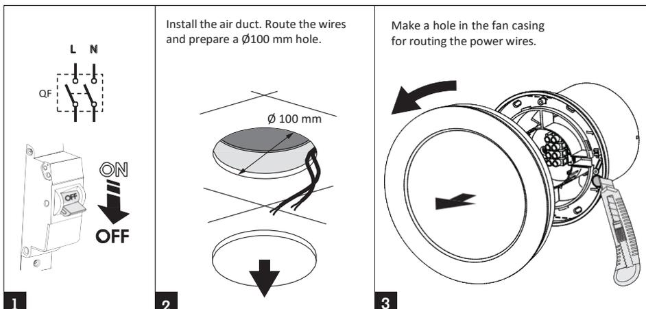
Connect the power supply unit and install it in a false ceiling. Route the wires through the hole in the casing and install the fan in the air duct.
